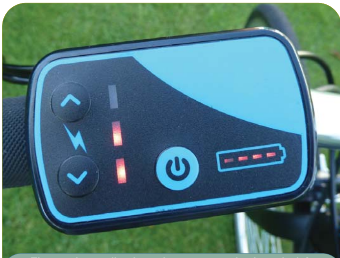
The speed controller shows three assistance levels on the left, with the rather ineffective fuel gauge on the right. This is the Upstart console - the Model T has a light switch at top right
