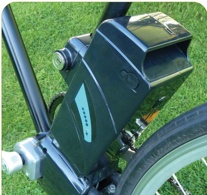
The discrete battery is modelled on the Panasonic crank-drive battery, but in this case the motor is in the front wheel
